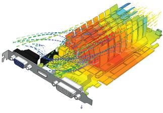
Surface temperatures and 3D particle plots can be used to assess the effectiveness of the new heatsink design.
