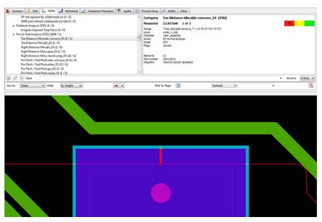
Valor DFM technology allows you to optimize your PCB design for manufacturing during the initial release process.
