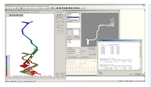
Use DC Drop analysis to prevent IC malfunction by identifying potential DC power-delivery issues such as excessive voltage drop.
