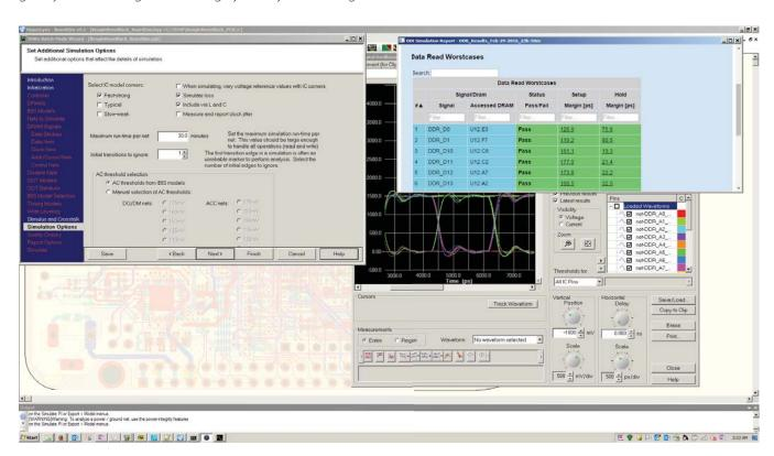
Advanced analysis in PADS includes a complete, integrated solution that allows verification of DDRx memory systems, making it easy to run full batch analyses for timing and SI.
