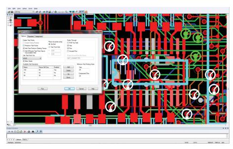
DFT audit reduces costly design iterations and ensures the testability of your designs before fabrication.
