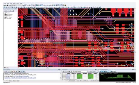
The Advanced PCB Option for PADS Standard Plus automatically adds accordion patterns for nets with length constraints.
