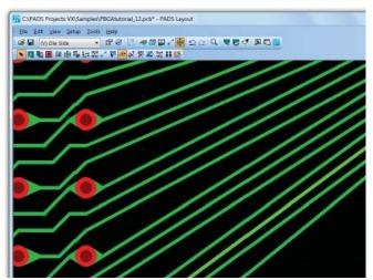
Interactive route editing supports any-angle routing to substrate pads, with or without a netlist.
