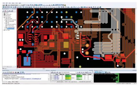
Automatically maintain differential pair rules including gap and length constraints.
