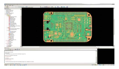
Perform design rule checks on boards for electro-magnetic interference and signal integrity issues with PADS HyperLynx DRC.
