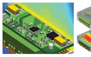
PADS FloTherm XT provides rapid thermal analysis of boards and packages.
