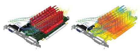
The surface temperatures on the PCB will quickly identify devices that are non-compliant with thermal specifications. Further understanding of the cooling performance can be achieved by examining the 3D flow field using the animated particle post-processing feature.
