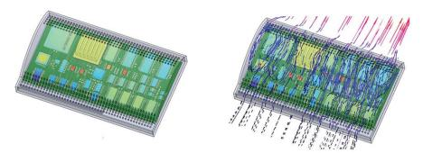
High-end graphics cards require novel cooling solutions – in this case, a heat sink with curved geometry has been designed to fit the enclosure. Surface temperatures and 3D particle plots can be used to assess the effectiveness of the new heat sink design.
